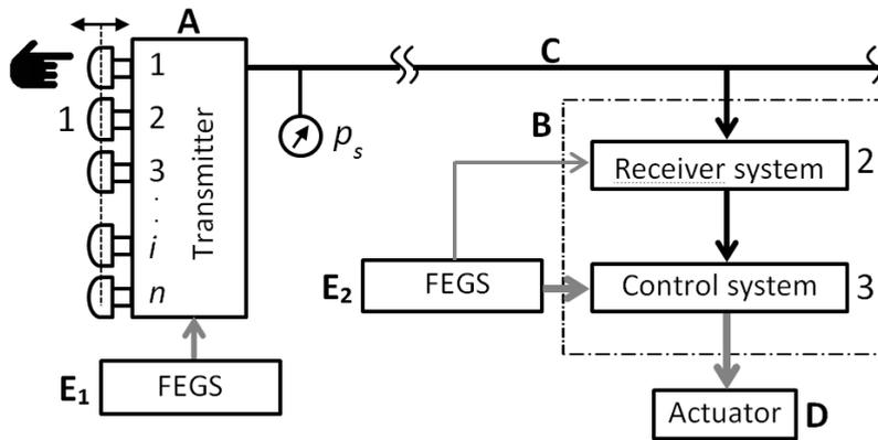
Fig. 1 General configuration of the proposed hydraulic control transmitter and receiver system: A, B – hydraulic transmitter and receiver, C – hydraulic signal line, D – actuator,  $E_{1,2}$  – fluid energy generation system, 1 – signal buttons, 2 – receiver system, 3 – control system,  $p_s$  – signal line pressure
