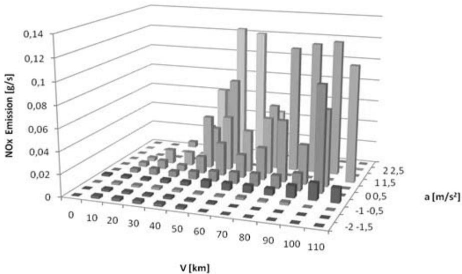
Fig. 9. Characteristics of the NO<sub>x</sub> emission in the range of vehiclespeed and acceleration during dynamic drive
