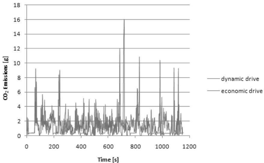
Fig. 16. The tracing of the second-by-second emission of CO<sub>2</sub> obtained during economic and dynamic drive
