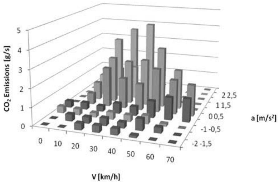
Fig. 11. Characteristics of the CO<sub>2</sub> emission in the range of vehiclespeed and acceleration during economic drive
