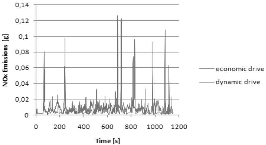
Fig. 18. The tracing of the second-by-second emission of NO<sub>x</sub> obtained during economic and dynamic drive
