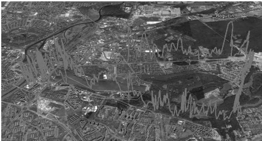
Fig. 4. Results of the CO<sub>2</sub> emissions during dynamic drive
