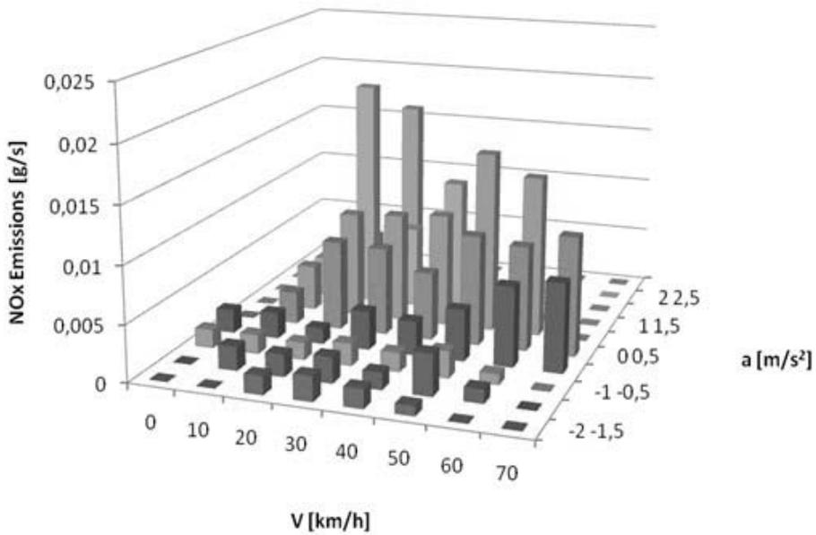
Fig. 15. Characteristics of the NO<sub>x</sub> emission in the range of vehiclespeed and acceleration during economic drive
