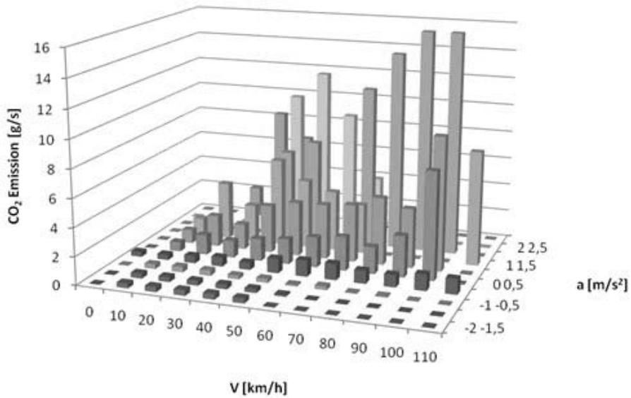
Fig. 5. Characteristics of the CO<sub>2</sub> emission in the range of vehiclespeed and acceleration during dynamic drive
