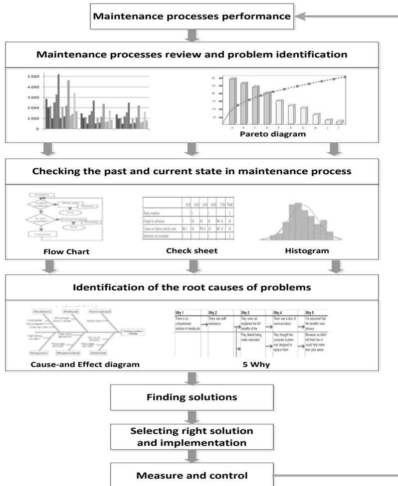
Fig. 8. Quality tools for maintenance process improvement
