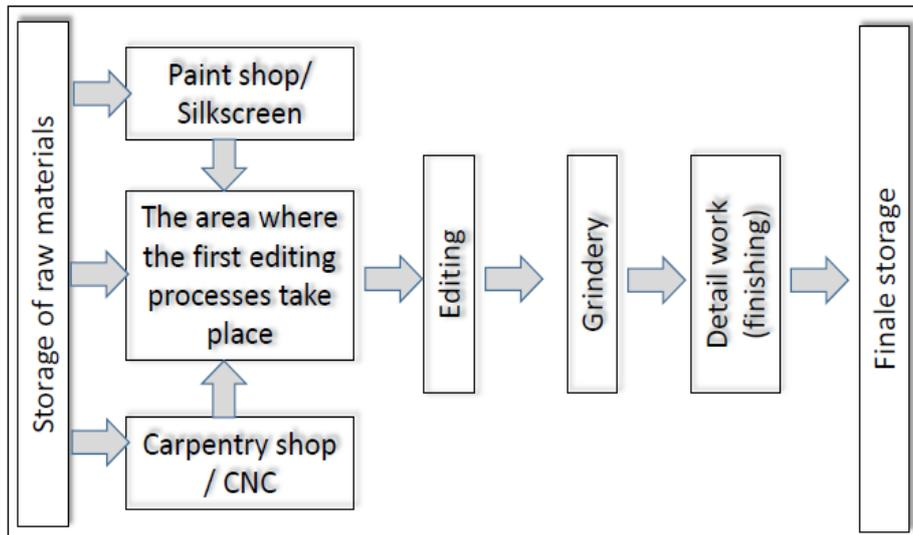
Fig. 1. Simplified scheme of the material flow
