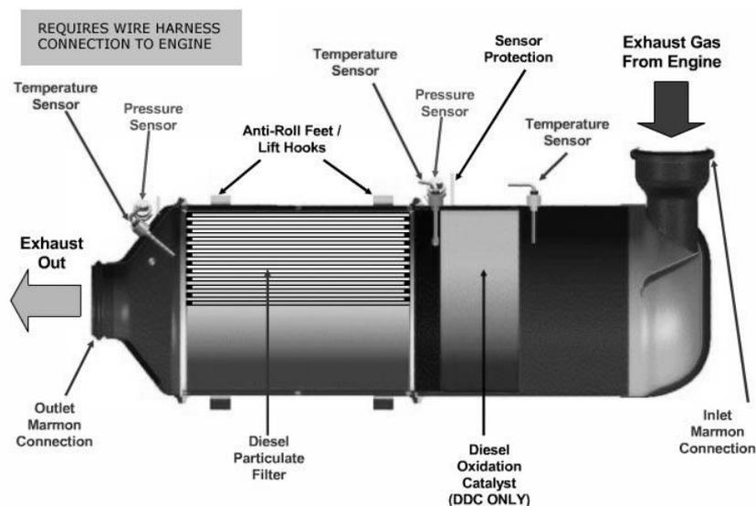
Fig. 4. The diagram of a purification system of exhaust gases from CI engines [11]
