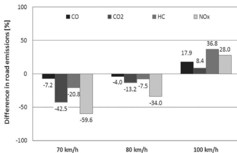
Fig. 3. Difference in emissions in a relation to the variable speed of vehicles [3]
