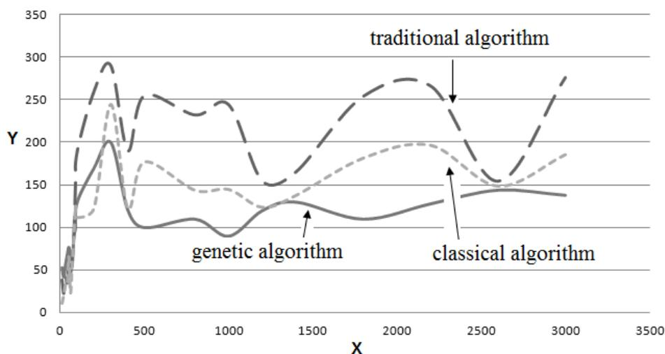
**Fig. 3** The graph showing the average time a driver has to spend to cross the crossroads depending on working time of the genetic algorithm based system and the classical system. Y- the average time of going through the intersection in seconds, X- system working time in minutes, Source: Elaboration of one's own
